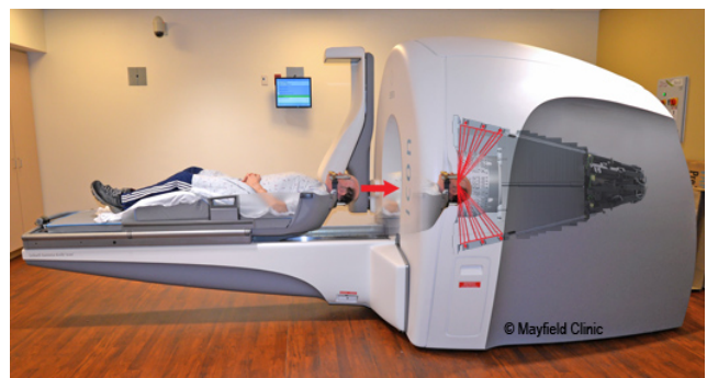
Figure 3. During radiosurgery, the patient lies on the table with their head held perfectly still with either a head frame or facemask in the treatment field. This photo shows Gamma Knife radiosurgery delivered through 192 openings in the machine.
